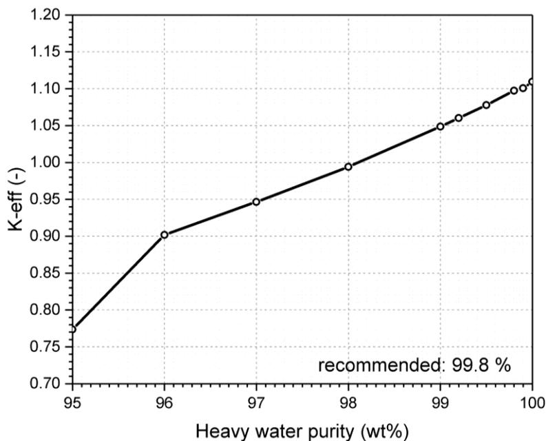
Figure 4: The results of different heavy water purity.
