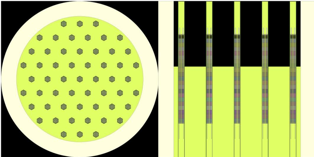
Figure 6: TEPLATOR DEMO core with 55 fuel assemblies in hexagonal lattice.
