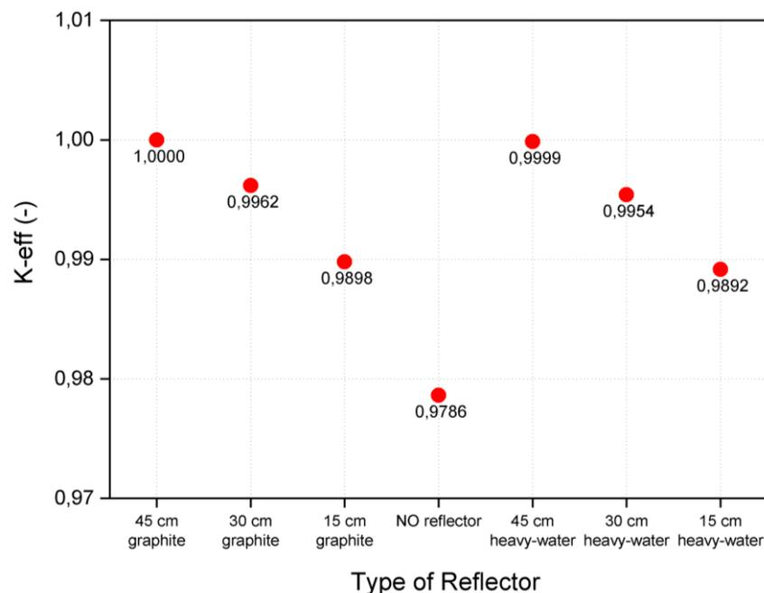
Figure 5: The results for different types of reflector and thicknesses.
