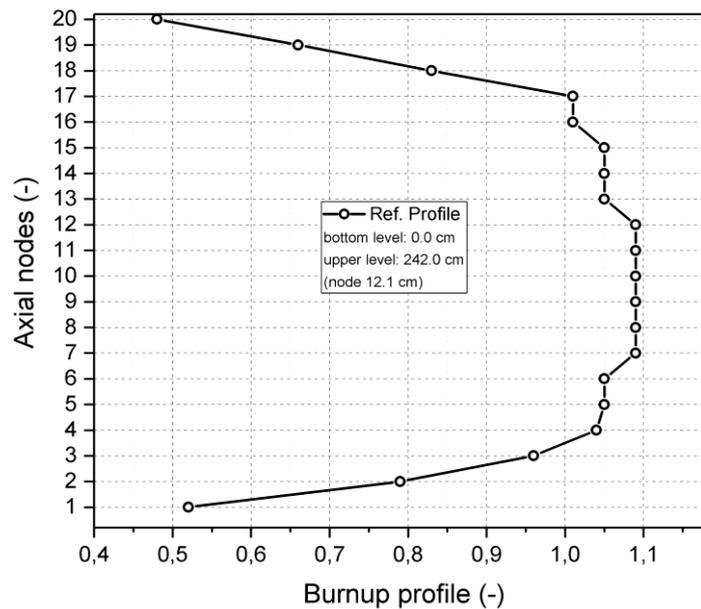
Figure 2: Axial burnup profile for VVER-440 spent nuclear fuel. [7]
