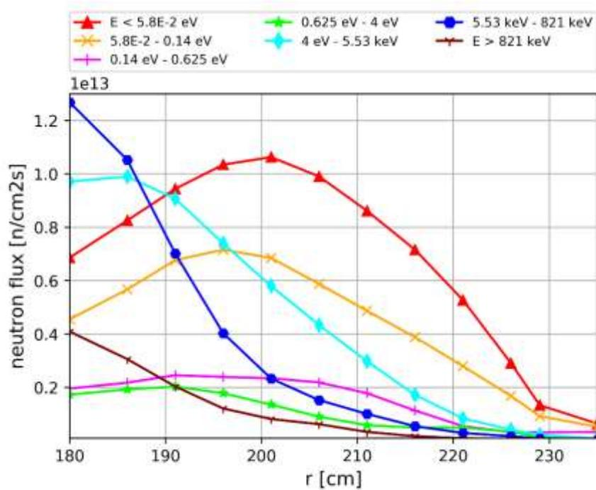
Figure 6: Detector D1 – Radial neutron flux – 7-group energy
