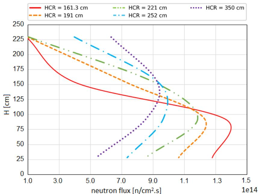
Figure 8: Effect of the moderator level on axial neutron flux profile distribution – 1. group thermal neutrons
