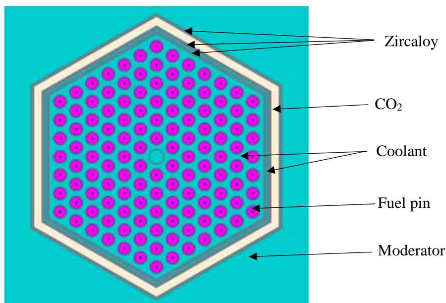
Figure 2: The composition of the fuel channel
