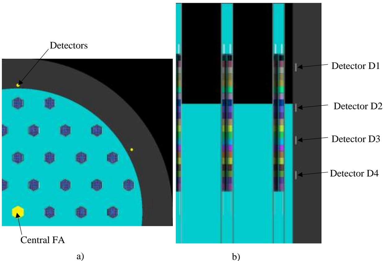
Figure 7: a) 60° symmetry of the detectors b) Axial position of the ex-core detectors
