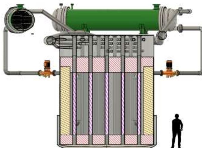
Figure 1: Schematic of the TEPLATOR – side view
