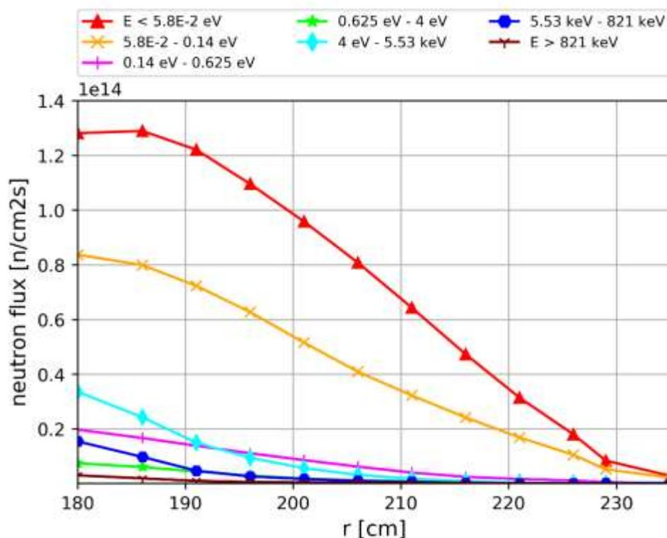
Figure 4: Radial neutron flux, 7-group energy structure, detector in the middle of the fuel assembly height under the moderator level
