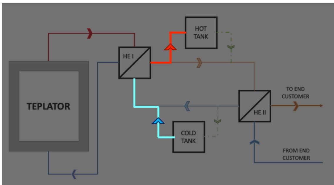
FIG. 5 Residual heat removal from TEPLATOR (charging of TES)
