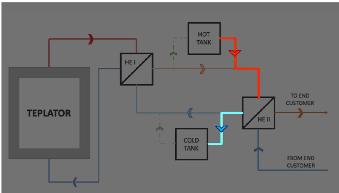
FIG. 6 Supplying heat to tertiary circuit from TES (discharging TES)
