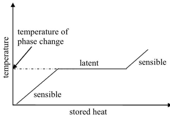
FIG. 3 Sensible and latent heat mechanism [2]
