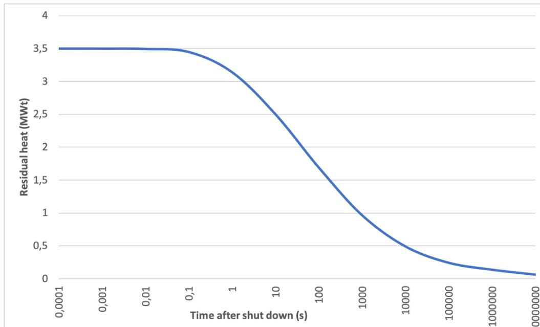
FIG. 4 Residual heat removal curve for TEPLATOR DEMO
